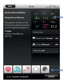
This area provides access to vital sign adjustment. Users may touch on any of the 6 diagnostic/monitoring topics and make adjustments. Adjustments here are temporary and the device will default to normal upon exit.
